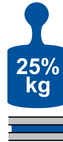
Horizontally mounted = 25% quoted load rating
