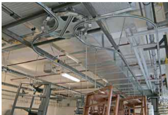
Suspension track system on a beach chair production line. Delivery to painting plant. Use of rotating and fall switches.
