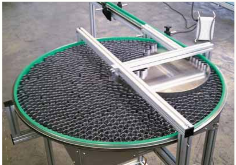
Buffer zone, as connection to belt conveyor.
