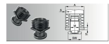
One-piece external body with injection-moulded thread. Octagonal screw head (except 0602020 + 0602222, hexagonal) Axial load capacity: M10 = approx. 100 kg / M16 = approx. 150 kg / >M22 = approx. 300 kg
