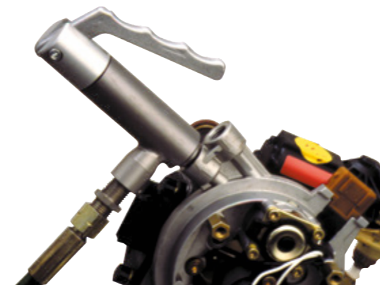
TW17H | Testing of injection pumps
