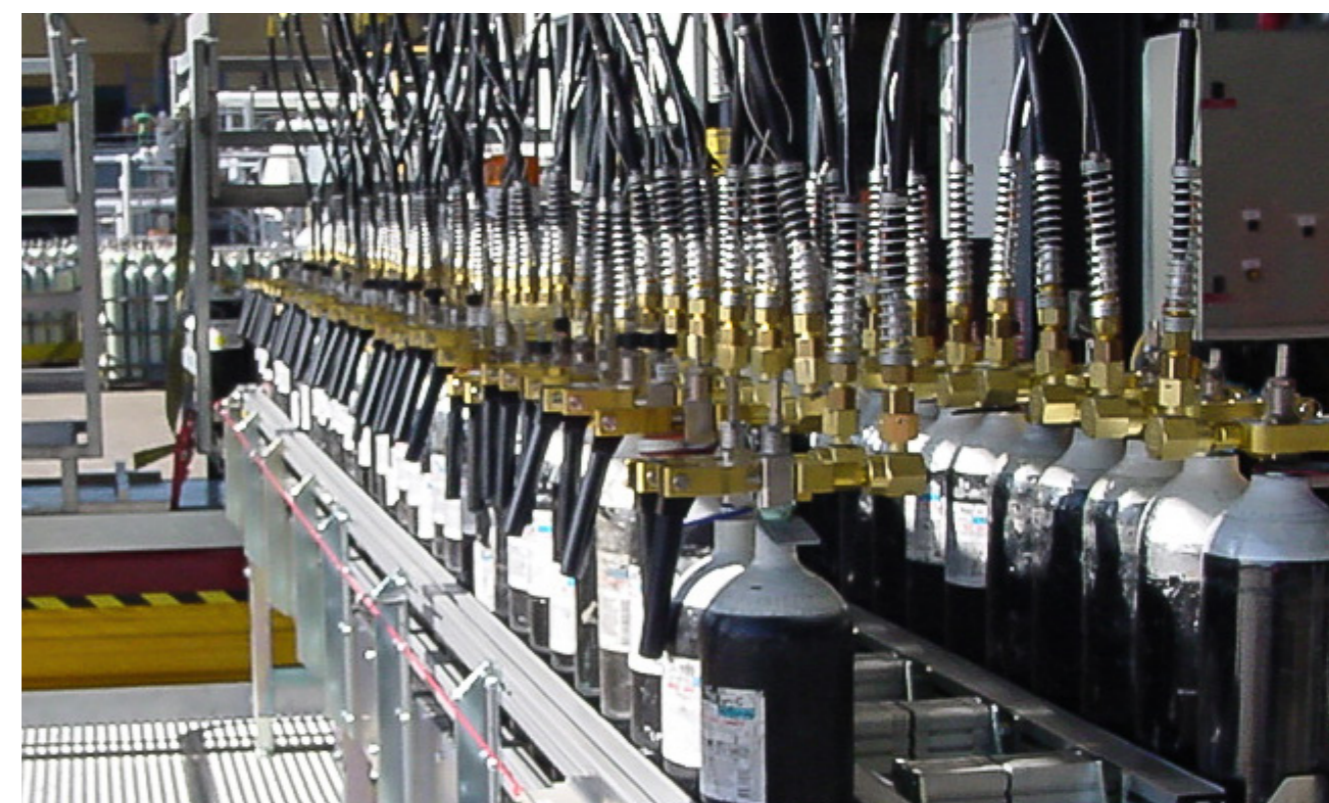
WEH® TW42 for medical oxygen applications with Pin-Index connection
