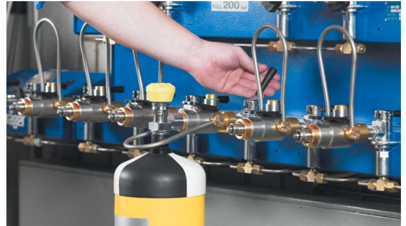
Existing BA cylinder filling rig after it has been upgraded to using the CLICKMATE® TW154
