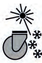
Overload caused by thermal effects
