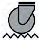
Overload caused by uneven surfaces
