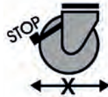
Overload caused by movement when in a locked position
